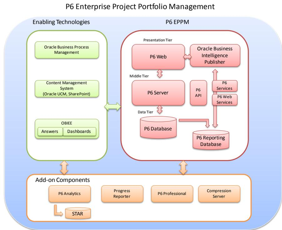
Typical P6 EPPM deployments consist of the following components:
